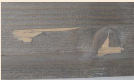
Surface finished with wood filler on dipped wood
