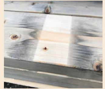
Dipping liquid does not reach all surfaces
