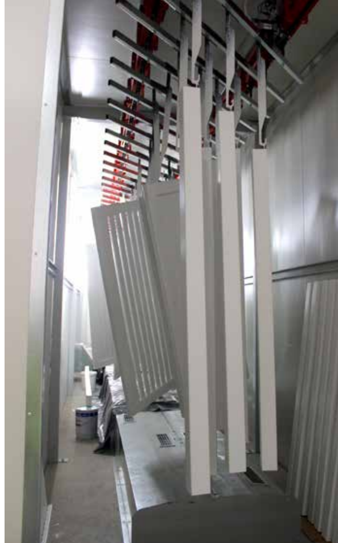
Painted products in drying chamber
